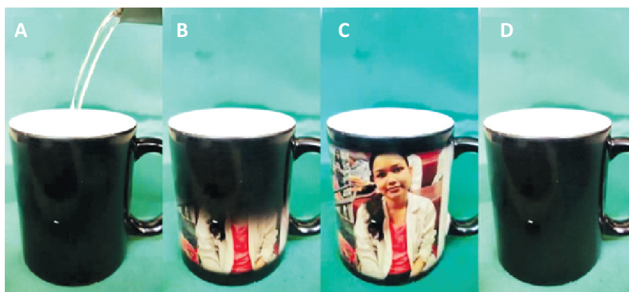
Fig. 1 : Demonstration of pigment change in a thermochromic cup, on exposure to hot liquid. From left to right - A-Hot water poured into a thermochromic cup, B - Gradual colour change in the exterior of the cup, C - Cup while retaining the hot water, D - Transition back to the initial colour once the water is at room temperature.
