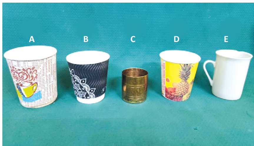
Fig. 2 : Cups of various materials tested in this study. From left to right - A-corrugated paper cup, B - jacketed paper cup, C - metal cup, D - wax-coated paper cup, and E - ceramic cup.
